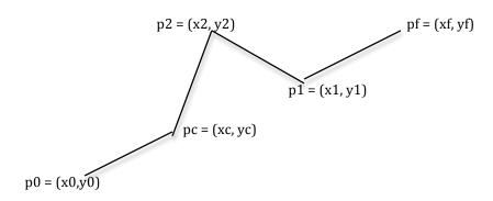
Given a center of rotation, (xc, yc), rotate another point (x1, y1) by  $\Theta$  degrees, the equations for the new point (x2, y2) are given above. See <a href="http://stackoverflow.com/questions/12161277/how-to-rotate-a-vertex-around-a-certain-point">http://stackoverflow.com/questions/12161277/how-to-rotate-a-vertex-around-a-certain-point</a>
